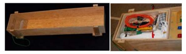
I also built a box to fill the space at the one end of the case and hold the electronics, bolts, Go-No Go Box and my four test cars along with a set of Grand Prix pennants. The box is 24"x14 3/4"x4", that makes the usable part 3 1/4" deep. The back is recessed to allow clearance of the hinges and bolt on the start gate and legs.
