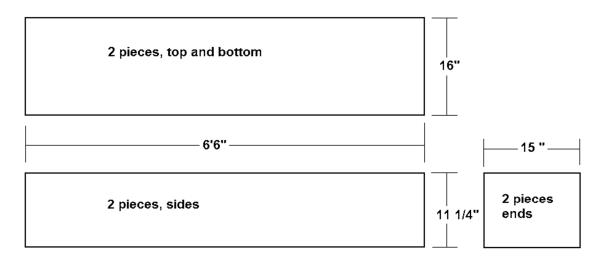
I simply glued the plywood together and shot brads to hold it all together. OK so I would not want to attach handles to the plywood and trust it to hold the weight of the track, but that is what the reinforcing 2x4's are for anyway. So far I just lift it from the bottom or by the 2x8's anyway.
